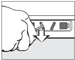
Use a screwdriver to push the emergency door latch downwards (see illustration). The drum door will open.
